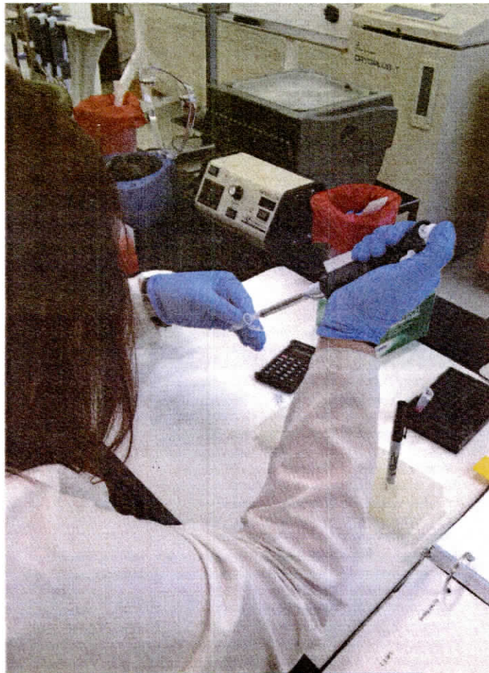
A student at the BioTechnical Institute of Maryland learns how to use a micropipette to accurately measure liquid volumes as small as one millionth of a liter.
